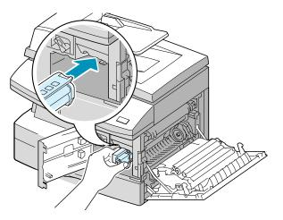
**5** Remove the starter toner cartridge from its bag. Gently shake the cartridge to loosen the toner.
